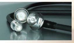
LISCA cable assemblies are specially developed for applications where low VSWR and low attenuation combined with low intermodulaiton products are required. The excellent performance is achieved by utilizing corrugated cables with low intermodulation designed connectors and a controlled assembly process with HUBER+SUHNER solder technology.
