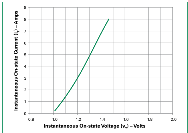
Figure 2: On-state Current vs. On-state Voltage (Typical)
