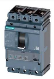
CIRCUIT BREAKER 3VA2 IEC FRAME 250 BREAKING CAPACITY CLASS H ICU=85KA @ 415 V 3POLE, LINE PROTECTION ETU330, LIG, IN=160A OVERLOAD PROTECTION IR=64A ...160A SHORT CIRCUIT PROTECTION II=1,5...12 X IN GROUNDFAULTPROTECTION IG=0,2... 1 X IN, TG=0,1/0,3MS BUSBAR CONNECTION
