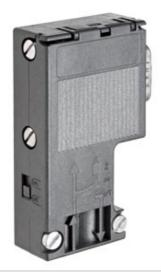
PROFIBUS bus connector, RS485, screw, without PG socket, 90° PROFIBUS bus connector, RS485, screw, without PG socket, 90° SIMATIC DP, BUS CONNECTOR FOR PROFIBUS UP TO 12 MBIT/S 90 DEGREE ANGLE OUTGOING CABLE, 15,8 X 64 X 35,6 MM (WXHXD), TERMINAT. RESIST. WITH ISOLAT. FUNCTION, WITHOUT PG SOCKET
