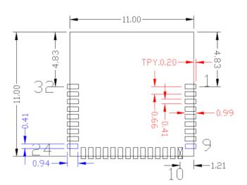
Figure 5. Module Pad Location from Origin
