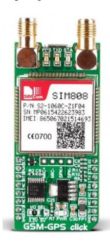
GSM-GPS click is a mikroBUS add-on board with a <u>SIM808</u> module that combines GSM/GPRS and GPS into a single device. Ideal for remote tracking devices in any shape or form.
