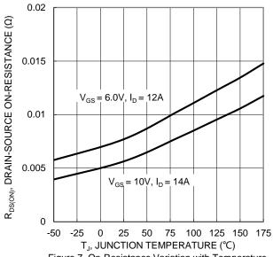
Figure 7. On-Resistance Variation with Temperature
