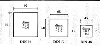
DIN 48 can be slot mounted using the standard fixing clip. DIN 72 & DIN 96 can be supplied with special fixing clips for slot mounting.
