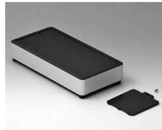
EE203059 SYNERGY E200 Aluminium AlMgSi 0,5 matt eloxiert 200x100x40mm IP 40
