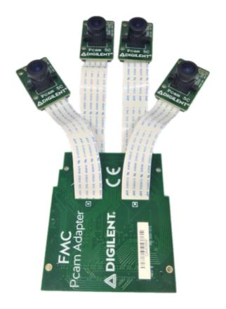
Figure 1. Four Camera Connection
