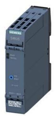
Thermistor motor prot. relay Standard evaluation unit 22.5 mm enclosure Spring-type terminals 2 CO contacts US = 24 V AC/DC Manual/Remote RESET with ATEX certification 2 LEDs (READY/TRIPPED) Galvanic separation Test/Reset button Open-circuit monitoring Short-circuit monitoring
