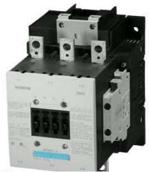
CONTACTOR, 275A/AC-1, AC(40...60HZ)/DC OPERATION UC 200...220V AUXIL. CONTACTS 2NO+2NC 3-POLE, SIZE S6 BAR CONNECTIONS CONVENT. OPERATING MECHANISM
