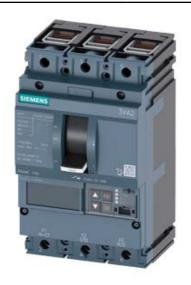
CIRCUIT BREAKER 3VA2 IEC FRAME 160 BREAKING CAPACITY CLASS M ICU=55KA @ 415 V 3POLE, LINE PROTECTION ETU560, LSIG, IN=160A OVERLOAD PROTECTION IR=64A ...160A SHORT CIRCUIT PROTECTION ISD=0,6..10X IN, II=1,5...10X IN NEUTRAL PROTECTION OPTIONAL WITH EXT. CT,UPTO 160% GROUNDFAULT, SWITCHABLE IG=0,2... 1 X IN, TG=0,050,8MS CABLE CONNECTION
