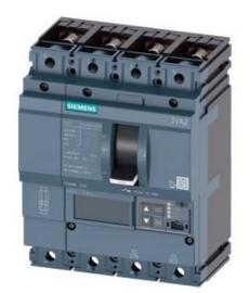
CIRCUIT BREAKER 3VA2 IEC FRAME 250 BREAKING CAPACITY CLASS H ICU=85KA @ 415 V 4POLE, LINE PROTECTION ETU550, LSI, IN=160A OVERLOAD PROTECTION IR=64A ...160A SHORT CIRCUIT PROTECTION ISD=0,6..10X IN, II=1,5..12X IN NEUTRAL PROTECTION ADJUSTABLE (OFF, UPTO 160%) BUSBAR CONNECTION
