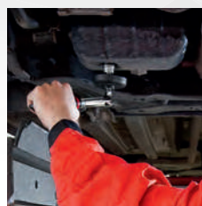
1 Drain plug unlocking in power position.
