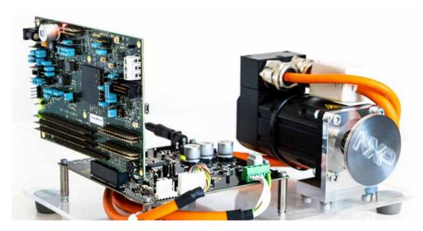
Expanding on the highly integrated MPC5775E microcontroller, the MCSPTR2A5775E motor control kit enables complex electric motor drive in the most efficient way for application targeting up to ISO 26262 ASIL D
