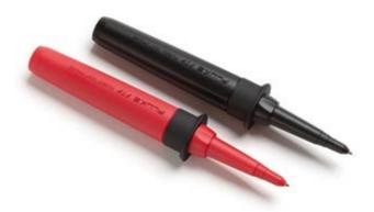
SureGrip Fused Test Probes with built-in replaceable fuses for additional measurement protection. If the probe fuse does blow, these fused test probes will still allow the meter to indicate live voltage, helping to prevent a possible misreading of no voltage present. These modular probes mount onto any standard modular test leads, for instance the Fluke TL221, TL222, or TL224. Rated to CAT III 1000V, these probes have removable tip guards for reduced probe tip exposure.
