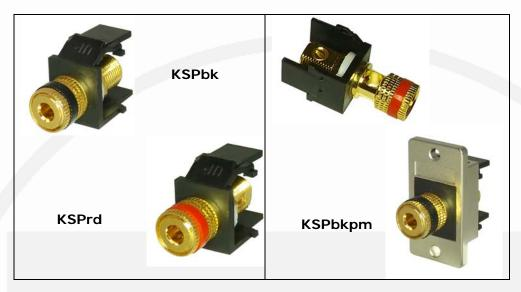
Keystone speaker connectors provide an easy solution for distributing audio signals within office or work area. These gold plated binding post connectors are designed for a quick screw-on or plug-in cable termination and the keystone adaptors provide an easy snap-in mounting into a keystone patch panel.
