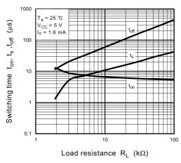
Fig. 11.15 Switching Time - RL
