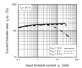
Fig. 11.12 I<sub>C</sub>/I<sub>F</sub> - I<sub>F</sub>
