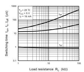
Fig. 11.14 Switching Time - RL
