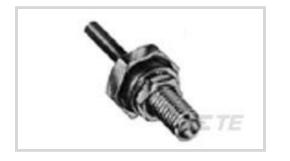
RF Interface: **SSMA** RF Connector Style: **Jack** RF Connector Mated Outer Diameter (Approximate): **7.24 mm [.285 in ]** Impedance: **50** Ω Compatible With RF Cable Type: **RG 405 Semi-Rigid**
