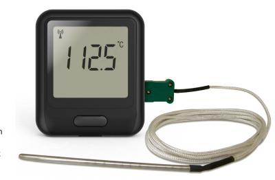
During configuration, the sensor will search for an existing wireless network whilst physically connected to the PC. It can then be placed anywhere within range of the network. If the sensor temporarily loses connectivity with the network, it will log readings until it is able to communicate again with the PC application or FilesThruTheAir™ Cloud (max 30 days at 10 second sample interval).
