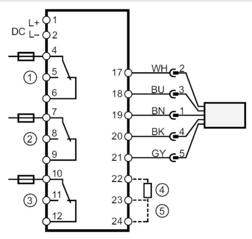
1 = Flow monitoring 2 = Wire monitoring 3 = Temperature monitoring 4 = Power-on delay time 5 = selection liquid/gas Note miniature fuse to IEC60127-2 sheet  $1 \le 5$  A fast acting Core colours : BN = brown BU = blue BK = black WH = white GY = grey
