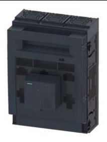
FUSE-SWITCH-DISCONNECTOR 3-POLE, NH2, 400A MOUNTING PLATE CONSTRUCTION COVER LEVEL 70 MM BOX TERMINAL FUSE MONITORING ELECTRONIC, EFM 10
