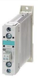
SEMI-COND. CONTACTOR 3RF2,1-PH. AC51 20 A 40 DEG. C 48-460 V / 4-30 V DC SCREW CONNECTION
