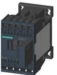
COUPLING RELAY, AC-3, 4KW/400V, 1NO, DC 24V, 0.85...1.85\*US, W. PLUGGED-ON VARISTOR 3-POLE SZ S00, SPRING-LOADED TERMINAL
