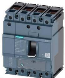
CIRCUIT BREAKER 3VA1 IEC FRAME 160 BREAKING CAPACITY CLASS N ICU=25KA @ 415 V 4-POLE, LINE PROTECTION TM220, ATFM, IN=100A OVERLOAD PROTECTION IR=70A ...100A SHORT CIRCUIT PROTECTION II=10 X IN NEUTRAL UNPROTECTED CABLE CONNECTION
