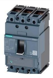
CIRCUIT BREAKER 3VA1 IEC FRAME 160 BREAKING CAPACITY CLASS S ICU=36KA @ 415 V 3-POLE, LINE PROTECTION TM220, ATFM, IN=100A OVERLOAD PROTECTION IR=70A ...100A SHORT CIRCUIT PROTECTION II=10 X IN BUSBAR CONNECTION
