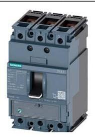
CIRCUIT BREAKER 3VA1 IEC FRAME 160 BREAKING CAPACITY CLASS N ICU=25KA @ 415 V 3-POLE, LINE PROTECTION TM220, ATFM, IN=40A OVERLOAD PROTECTION IR=28A ...40A SHORT CIRCUIT PROTECTION II=10 X IN BUSBAR CONNECTION
