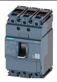
CIRCUIT BREAKER 3VA1 IEC FRAME 160 BREAKING CAPACITY CLASS N ICU=25KA @ 415 V 3-POLE, LINE PROTECTION TM210, FTFM, IN=16A OVERLOAD PROTECTION IR=16A FIXED SHORT CIRCUIT PROTECTION II=10 X IN CABLE CONNECTION
