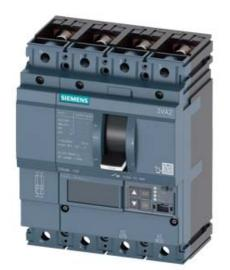
CIRCUIT BREAKER 3VA2 IEC FRAME 100 BREAKING CAPACITY CLASS C ICU=110KA @ 415 V 4POLE, LINE PROTECTION ETU850, LSI, IN=100A OVERLOAD PROTECTION IR=40A ...100A SHORT CIRCUIT PROTECTION ISD=0,6..10X IN, II=1,5..12X IN NEUTRAL PROTECTION ADJUSTABLE (OFF, UPTO 100%) BUSBAR CONNECTION
