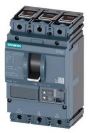
CIRCUIT BREAKER 3VA2 IEC FRAME 100 BREAKING CAPACITY CLASS H ICU=85KA @ 415 V 3POLE, LINE PROTECTION ETU550, LSI, IN=63A OVERLOAD PROTECTION IR=25A ...63A SHORT CIRCUIT PROTECTION ISD=0,6..10X IN, II=1,5..12X IN NEUTRAL PROTECTION OPTIONAL WITH EXT. CT,UPTO 160% CABLE CONNECTION
