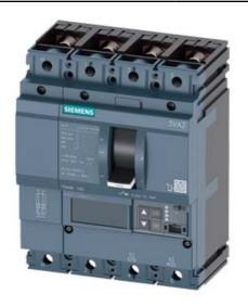
CIRCUIT BREAKER 3VA2 IEC FRAME 160 BREAKING CAPACITY CLASS C ICU=110KA @ 415 V 4POLE, LINE PROTECTION ETU860, LSIG, IN=100A OVERLOAD PROTECTION IR=40A ...100A SHORT CIRCUIT PROTECTION ISD=0,6..10X IN, II=1,5..12X IN NEUTRAL PROTECTION ADJUSTABLE (OFF, UPTO 160%) GROUNDFAULT, SWITCHABLE IG=0,2... 1 X IN, TG=0,050,8MS BUSBAR CONNECTION
