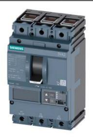
CIRCUIT BREAKER 3VA2 IEC FRAME 160 BREAKING CAPACITY CLASS H ICU=85KA @ 415 V 3POLE, LINE PROTECTION ETU860, LSIG, IN=40A OVERLOAD PROTECTION IR=16A ...40A SHORT CIRCUIT PROTECTION ISD=0,6..10X IN, II=1,5...12X IN NEUTRAL PROTECTION OPTIONAL WITH EXT. CT,UPTO 160% GROUNDFAULT, SWITCHABLE IG=0,2... 1 X IN, TG=0,050,8MS CABLE CONNECTION
