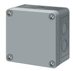
This level monitor for two electrodes preferrably serves to the limit control, e.g. as overflow or running dry protection of a conducting liquid. The device is integrated in a shock-resistant plastic housing of the type 94 and can also be used for outside-resp. waterproof mounting according to its protection system IP 54.
