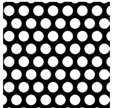
Ø5mm/ 0.196" Hole on 6.5mm/ 0.256" x 60° Pitch 53.7% Free Area
