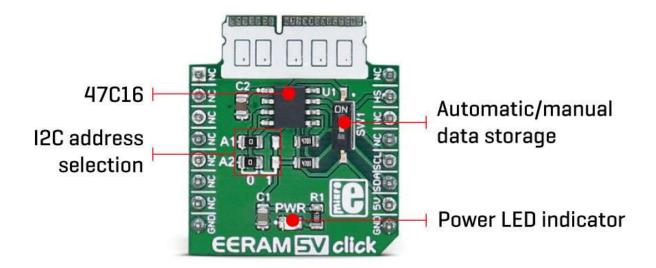
The EERAM 5V click can backup or restore its content, utilizing the integrated EEPROM non-volatile array, which is not directly accessible. There are several ways to achieve this:
