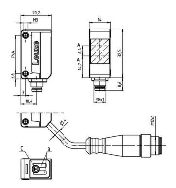
A Optical axis B Indicator diode
