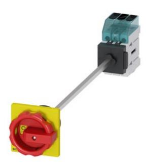
Switch disconnector 3LD3, main switch 3-polig, lu 16A operational switch at AC-23 A at 400 V 7,5 kW floor mounting Base mounting with door coupling center-hole 22,5 mm rotary operationg mechanism red/yellow  $66 \times 66$  mm
