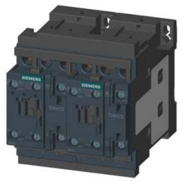
REV. COMB. FOR 3RA27, AC3, 18.5KW/400V, DC24V 3-POLE, SZ S0 SCREW TERMINAL ELECTR. AND MECH. INTERLOCK 2NO INTEGR.
