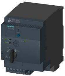
SIRIUS, COMPACT STARTER, REVERSING STARTER 690 V, 110 ... 240 V AC/DC, 50 ... 60 HZ, 1 ... 4 A, IP20, MAIN CIRCUIT CONNECTION: PLUG-IN, W/O TERMINALS, AUXILIARY CIRCUIT CONNECTION: SCREW TERMINAL
