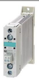
SOLID-STATE CONTACTOR 3RF2,1-PH AC51 20A / AC15 12A 40 DEGR. C 48-460V / 4-30V DC INSTANT. SWITCHING
