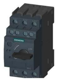
SPECIAL TYPE CIRCUIT BREAKER SIZE S0, FOR MOTOR PROTECTION, CLASS 10, A-RELEASE 27...32A, SHORT-CIRCUIT RELEASE 400A, SCREW TERMINAL, STANDARD SWITCHING CAPACITY, W. TRANSVERSE AUXILIARY SWITCH 1NO+1NC AMBIENT TEMPERATURE -50 DEGREES C 500 **SWITCHING CYCLES**
