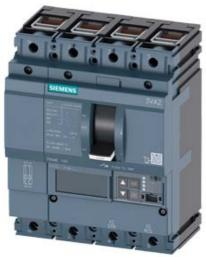
CIRCUIT BREAKER 3VA2 IEC FRAME 100 BREAKING CAPACITY CLASS H ICU=85KA @ 415 V 4POLE, LINE PROTECTION ETU550, LSI, IN=25A OVERLOAD PROTECTION IR=10A ...25A SHORT CIRCUIT PROTECTION ISD=0,6..10X IN, II=1,5..12X IN NEUTRAL PROTECTION ADJUSTABLE (OFF, UPTO 160%) CABLE CONNECTION
