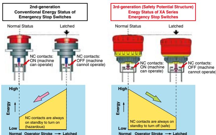
With XA emergency stop switches, the potential energy level of the latched status is lower than that of normal status. In the event the switch is damaged due to excessive shocks, the NC contacts will turn off, thus stopping the machine (patented).
