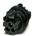
Circular connectors (cable-side), Contact insert, housing material: PPE, color: black, number of positions: 3, min. conductor cross section: 1.5 mm², max. conductor cross section: 6 mm², nom. voltage: 690 V AC, rated current: 35 A, Connection method: Screw connection, Type of contact: Pin
