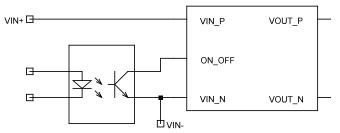
Figure T2. ON/OFF Control Circuit
