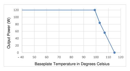
Fig. A-1: Derating Max Baseplate (115°C) Temperature, Vin = 24V (Tested on 10x10 inch PCB)
