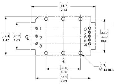
FOOTPRINT IS SAME AS STANDARD WITH **ADDITIONAL** COMPONENT **CLEARANCE FOR** FLANGED BASEPLATE
