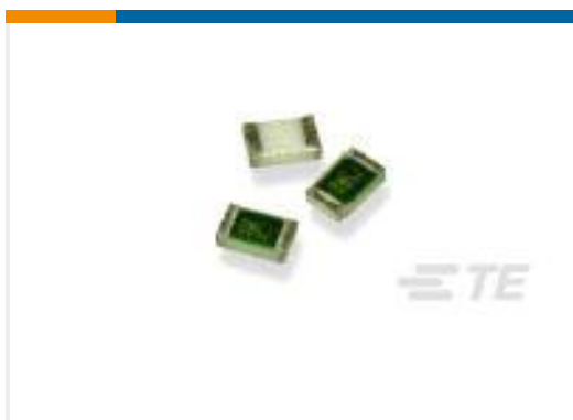
TE Part #9-1614882-8 CPF 0603 20R 0.1% 25PPM 1K RL
