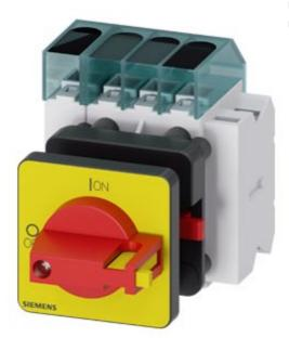
Switch disconnector 3LD3, main switch 3-polig + N, lu 25A operational switch at AC-23 A at 400 V 9,0 kW front mounted Base mounting with center-hole 22,5 mm knob-operated mechanism red/yellow 48 x 48 mm with auxiliary 1NO+1NC
