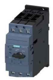
CIRCUIT BREAKER SIZE S2. FOR MOTOR PROTECTION, CLASS 20, A-RELEASE 20...25A, N-RELEASE 325A, SCREW TERMINAL, STANDARD BREAKING CAPACITY
