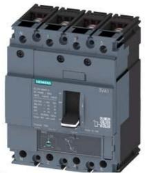
CIRCUIT BREAKER 3VA1 IEC FRAME 160 BREAKING CAPACITY CLASS M ICU=55KA @ 415 V 4-POLE, LINE PROTECTION TM220, ATFM, IN=20A OVERLOAD PROTECTION IR=14A ...20A SHORT CIRCUIT PROTECTION II=10 X IN NEUTRAL PROTECTION 100% BUSBAR CONNECTION
